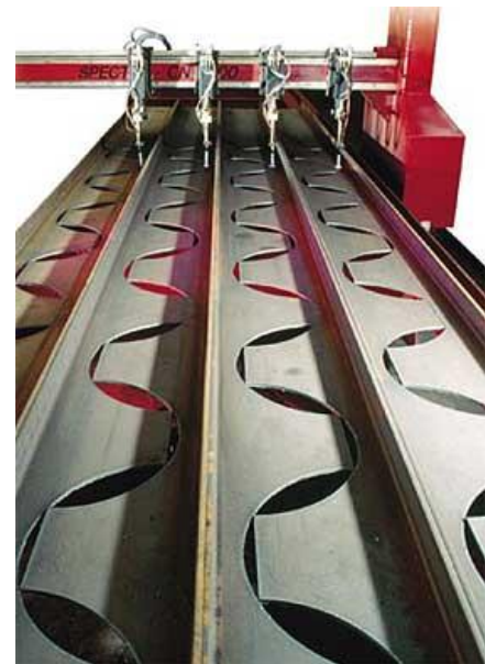
Figure 1.6: Cellular Beam Fabrication
